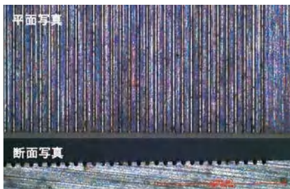
微細溝入り試験片 溝深さ0.03×溝幅0.03
